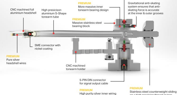
Stainless steel counterweight sliding on a high precision thread on two TPE rings for damping. This design enables better stability and a finer range of motion to set tracking force with increased accuracy.
